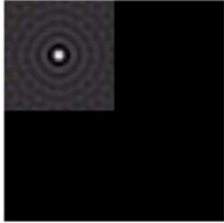
FIGURE 4.39 Padded lowpass filter in the spatial domain (only the real part is shown).
