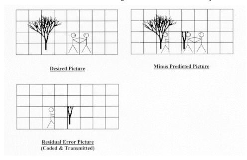
**Final Motion Estimation Prediction:** Not every macroblock search will result in an acceptable match. If the encoder decides that no acceptable match exists (again, the "acceptable" criterion is not MPEG defined, and is up to the system designer) then it has the option of coding that
